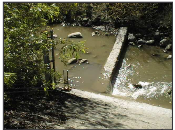
Figure 3.3: Two of the four gauging locations on Carpinteria Creek, 8 th Street Footbridge and the USGS station near Hwy 192 Bridge. Both have staff gauges at the deepest point of the channel at a determined cross-section.
