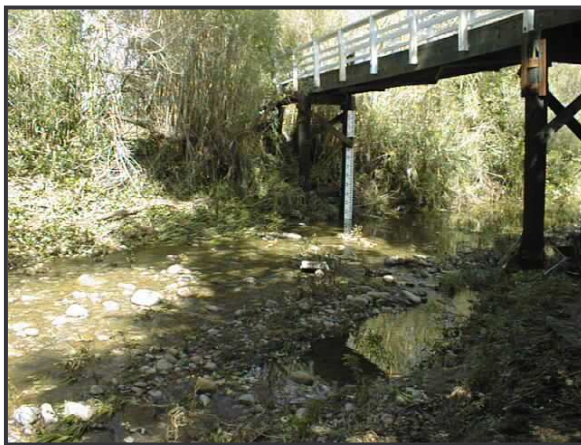
Figure 3.3: Two of the four gauging locations on Carpinteria Creek, 8 th Street Footbridge and the USGS station near Hwy 192 Bridge. Both have staff gauges at the deepest point of the channel at a determined cross-section.
