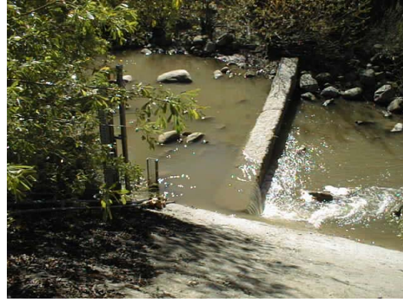
Figure 2: Two of the four gauging locations on Carpinteria Creek, 8 th Street Footbridge and the USGS station near Hwy 192 Bridge. Both have staff gauges at the deepest point of the channel at a determined cross-section.
