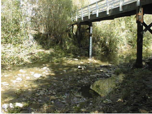
Figure 2: Two of the four gauging locations on Carpinteria Creek, 8 th Street Footbridge and the USGS station near Hwy 192 Bridge. Both have staff gauges at the deepest point of the channel at a determined cross-section.
